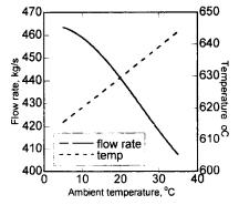
Fig. 5 Variations of the flow rate and temperature of exhaust gas of the gas turbine with ambient temperature
