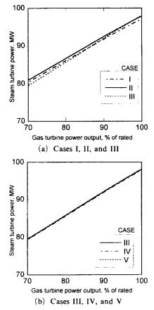
Fig. 6 Off-design performance of a steam turbine with gas turbine load
