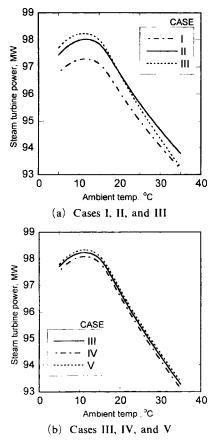
Fig. 4 Off-design performance of a steam turbine with ambient temperature
